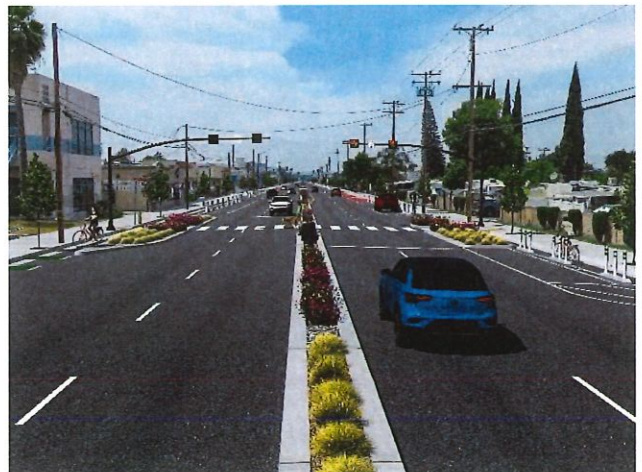
Photo 4: Rendering of proposed concepts including Class IV bicycle facility, High Intensity Activated Crosswalk (HAWK), and landscaped median
