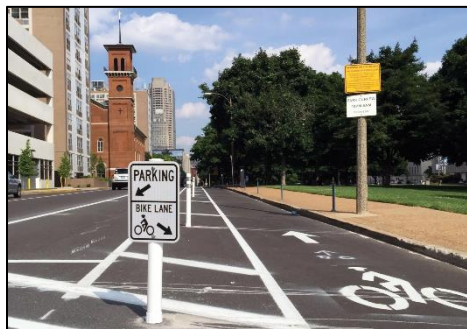
Photo 10 Class IV Bikeway with Parking (NACTO)
